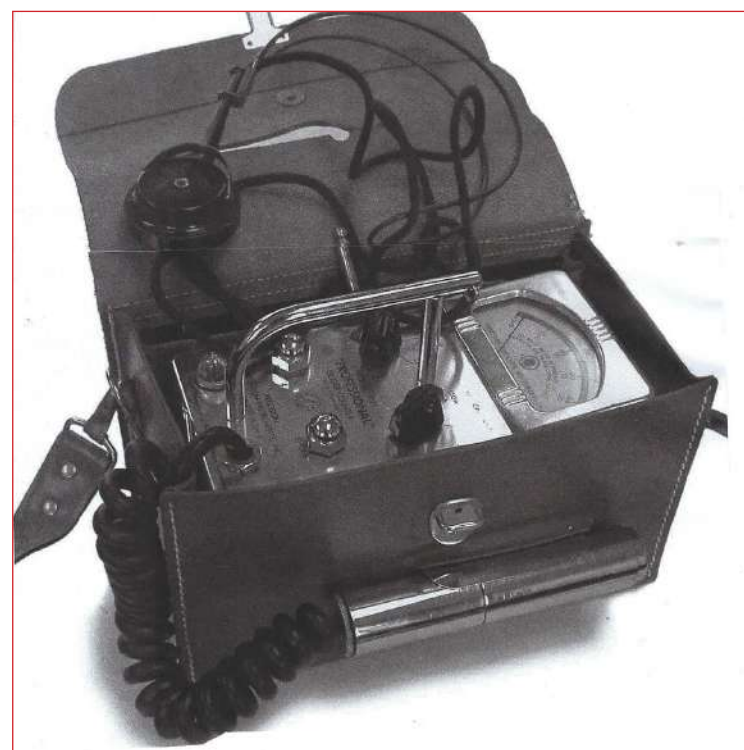
A model 1954 model professional Geiger Counter kit. Could be purchased at the Newell Airport and go out and make some "real money". Newell Museum
